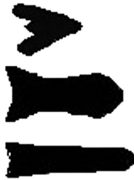
Figure 8. Shape of EFP as a function of velocity of detonation. TNT (top), Octal, 75/25 (middle), and HMX (bottom). Additional data are given in Table 3.
